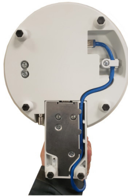
Cable Routing Under Scale
