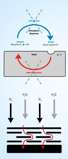
Corrosion is an electrochemical process that consists of cathodic and anodic reactions produced by electrons and ionic diffusion. Axalta coating technologies inhibit at least one of these reactions. The cathodic reaction is halted or reduced because the coating acts as a barrier; it markedly reduces the diffusion of the elements involved in the corrosion process  $(H_2O, O_2)$ .
