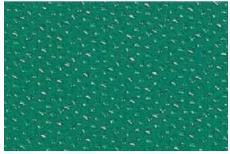
**Colorcoat HPS200\*** - this has a 'dimpled' surface texture, quite different from traditional leathergrain Plastisol. This Scintilla pattern has a tiny 'S' impressed inside it. It should be solvent washed with Xylene if weathered for less than one month.
