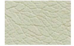
**Plastisol HP200\* -** easily recognised by its classic 'leathery' surface texture. It should be solvent washed using White Spirit if weathered for less than one month. Older, weathered surfaces only require cleaning/degreasing.
